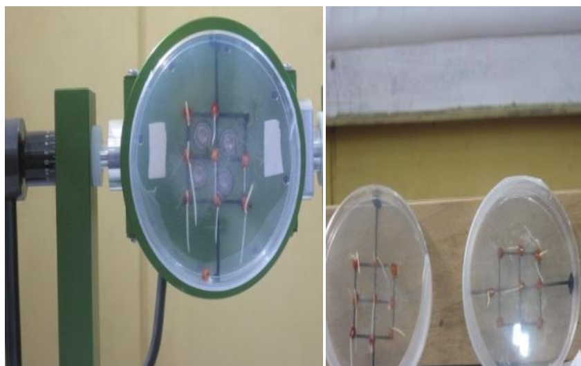
Fig. 1. Photograph of guinea corn seedlings in simulated microgravity and normal earth environments
