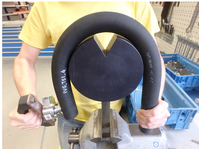
Figure 5. Measurement of radial reaction forces in the course of standard bending test.
