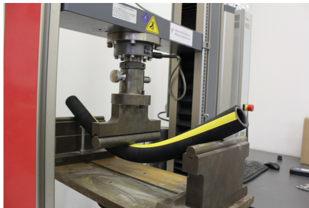
Figure 3. Three-point bending at a deflection of 80 mm.
