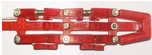
Figure 3. Fabricated prototype of the linkage finger mechanism.
