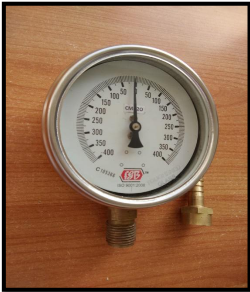
Fig. 1. Hand Held Pressure Manometer device (PIMax)
