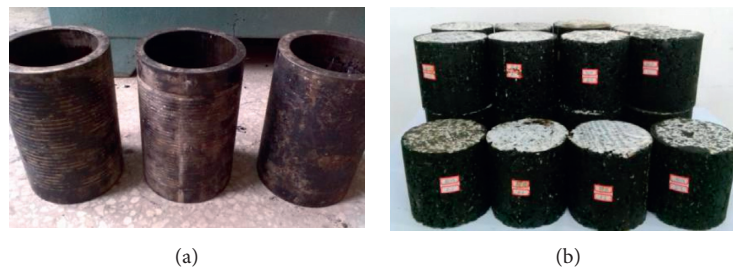
FIGURE 2: Sample making. (a) Molds used for testing the molded specimens. (b) Molded parts of the specimens.
