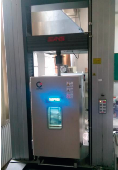
FIGURE 3: CMT5105 microcomputer-controlled electronic universal testing machine.
