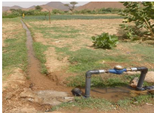
Fig. 6. Tachagor water quantification meter
