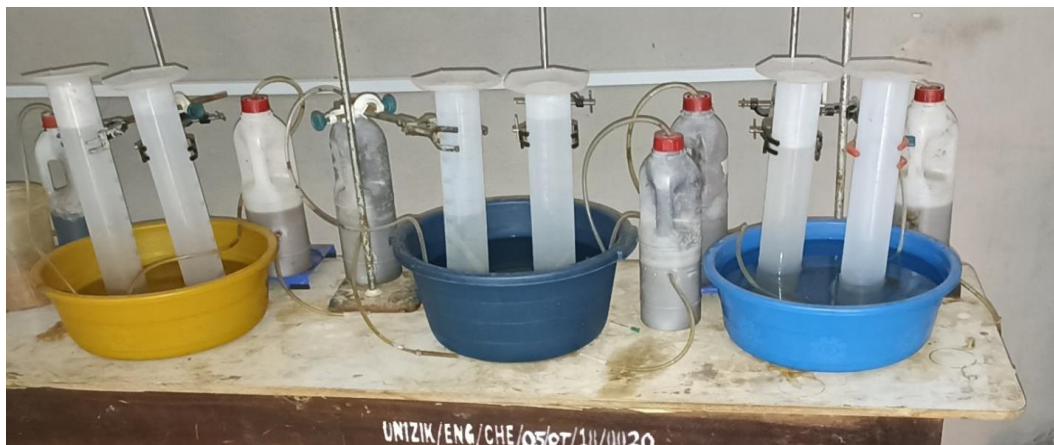
Fig. 1. The laboratory setup of anaerobic digestion
