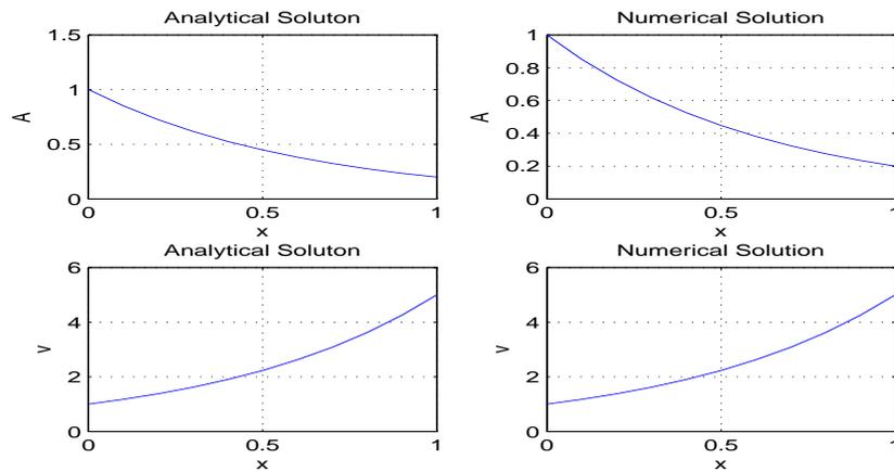
Fig. 2. Steady-state analytical and numerical solutions for velocity  $v$  and cross-sectional area  $A$  with  $h = 0.01$
