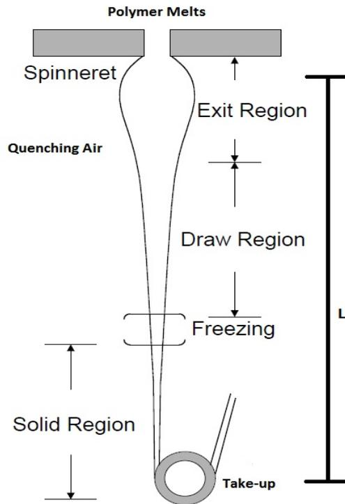
Fig. 1. Melt Spinning Process [2]
