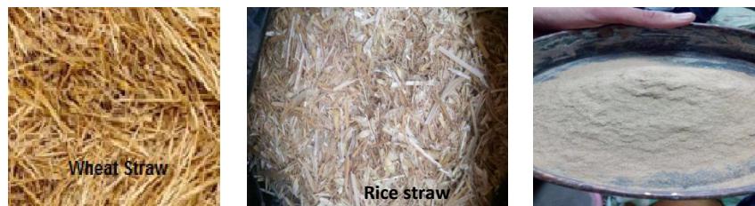
Fig. 2. Wheat and rice straw ash before and after grinding
