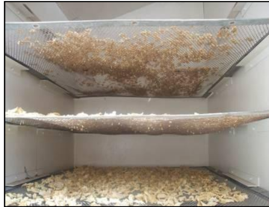
Fig. 6. Drying chamber rhizomes with three screens
