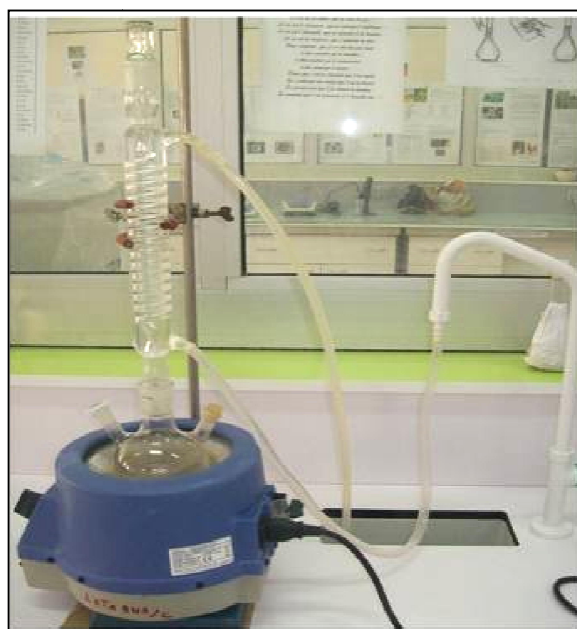
Fig. 9. Extraction device by refrigerant under reflux
