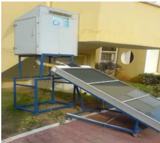
Fig. 5. Experimental setup: Indirect solar dryer
