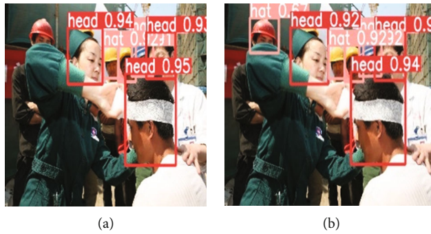
FIGURE 5: Improved mosaic result: a blocked helmet is detected in (b).
