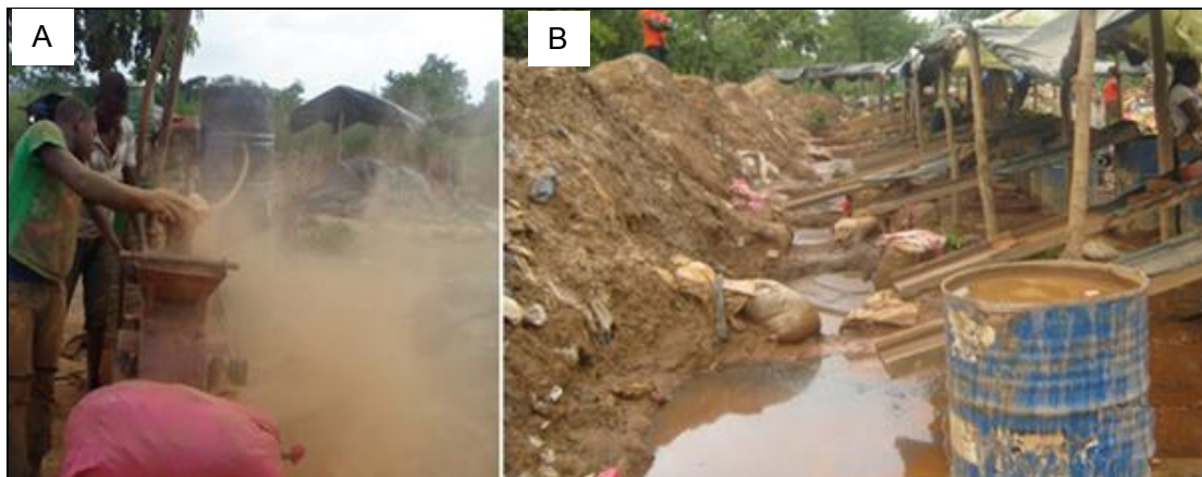
Fig. 10. Vein ore grinding (A) and washing (B) site by gold miners at Floleu
