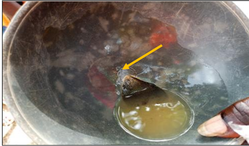
Fig. 8. Concentrate consisting of iron filings and gold powder obtained by washing the ore.
