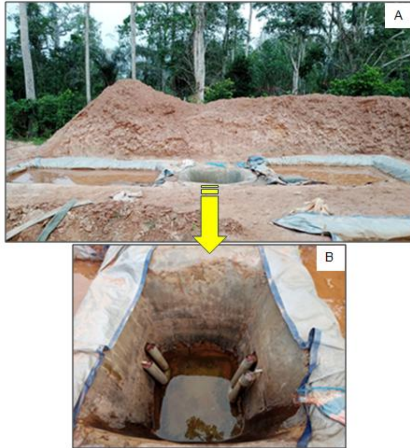
Fig.11. Device for treating gold with cyanide (A) and the interior of a hollow basin (B) at Floleu (in operation)
