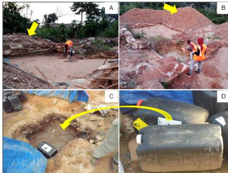
Fig. 15. Illustration of the fate of the waste from cyanidation sites identified in the study area; treatment residues (A), waste rock (B), chemical packaging (C and D)
