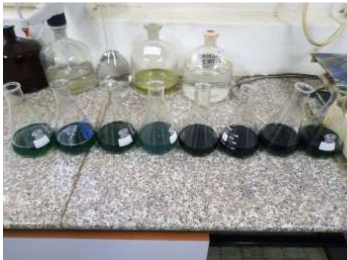
Figure 1. Endpoint of a reaction using orthophosphoric acid (4 at the left) and without using orthophosphoric acid (4 at the right) for similar soil sample.
